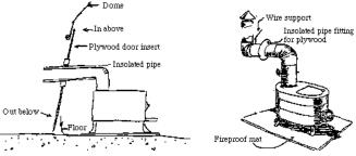
Attach a horizontal section of pipe to this elbow and pass this pipe through the wall such that it will slant slightly down towards the outside. This will keep rain from following the pipe and dripping inside your dome. We recommend using insulated stovepipe throughout. Place an elbow on the outside. Attach a vertical pipe on the outside pipe and a spark arrester cap
